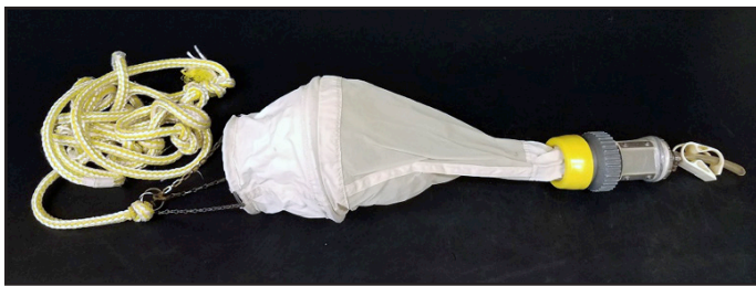
Figure 10. A Wisconsin-style plankton net captures a representative zooplankton sample and provides for both qualitative and quantitative analysis.
